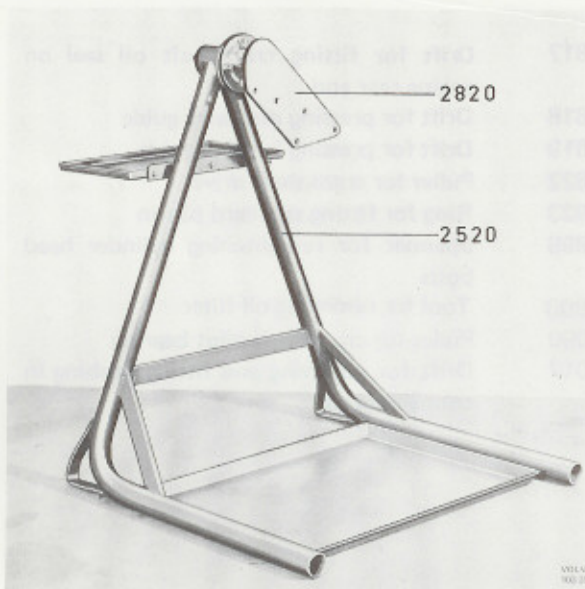
Fig. 20-3. Stand for engine 2520 Stand. Used together with fixture 2820
