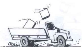
Reason: Over energetic braking out-of-round brake drums.
