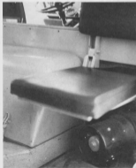
Separate fan air system for passengers and a flip-on cover over engine allows work from inside on sub-zero days.
